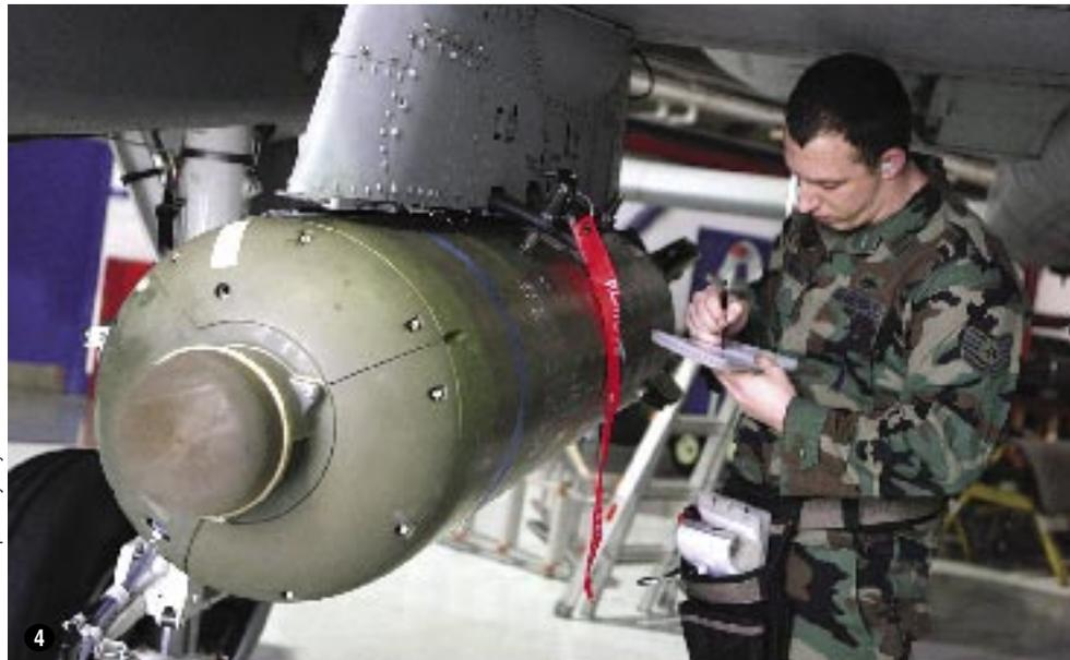
**[4]** TSgt. Anthony Tringler checks the paperwork as an inert cluster bomb dispenser is loaded on an A-10 pylon for training.
