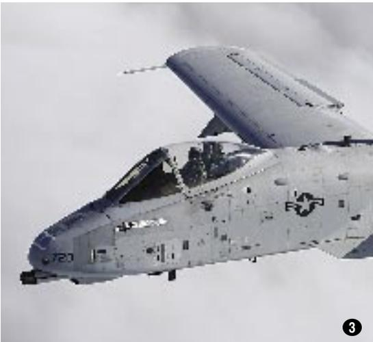
*[4] The Warthog's pilot is seated in an armored "titanium bathtub" that provides extra protection from small arms. The bulletproof canopy of diffusion-bonded acrylic offers further safety. [5] An A-10 shows off its belly and "false canopy" painted underneath. The optical trick is meant to keep enemies wondering about what the aircraft is about to do.*
