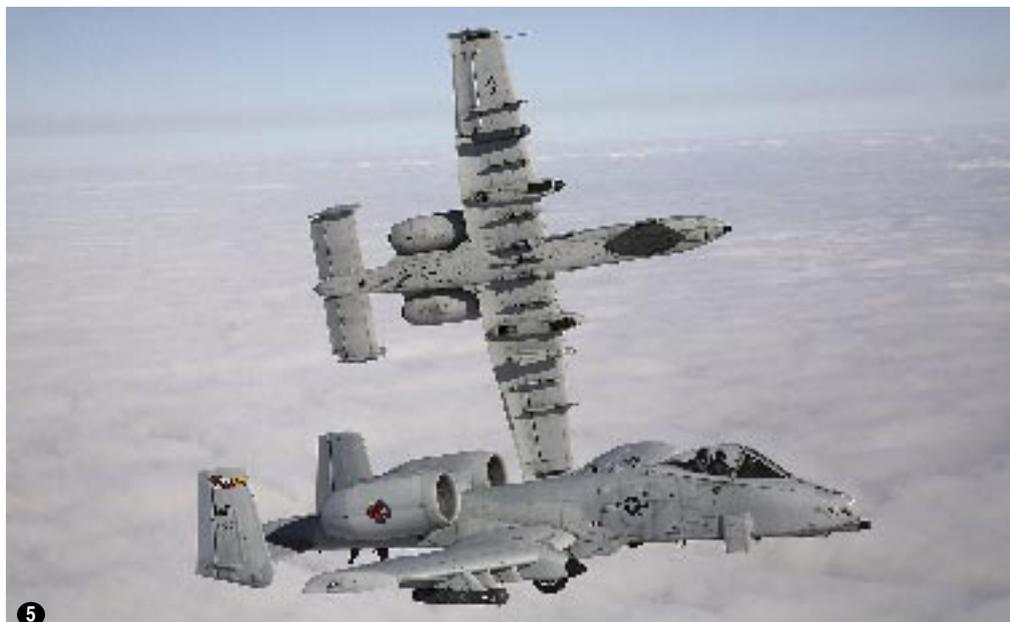
**[1]** Lt. Chris Cisneros adjusts his earplugs on the noisy Martin State Airport flight line. **[2]** The A-10C upgrade gives the aircraft the ability to use advanced targeting devices such as the Litening pod carried here on the outboard right wing. The pods provide detailed target images from long distance, and also full-motion video feeds to a command center if desired.
